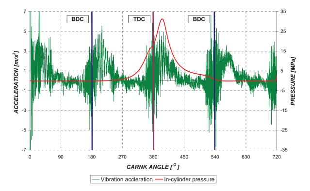
*Fig. 3. Traces of fourth cylinder pressure and vertical vibration for engine fuelled by petrol (rpm=1500, full load)*
