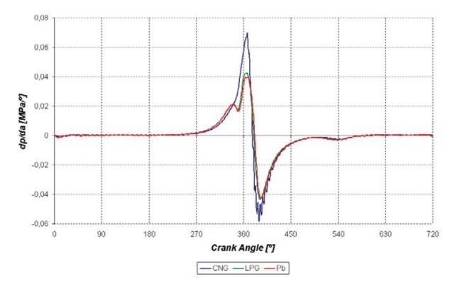
Fig. 2. Combustion hardness traces for all kind of fuels (2000 rpm, full load)
