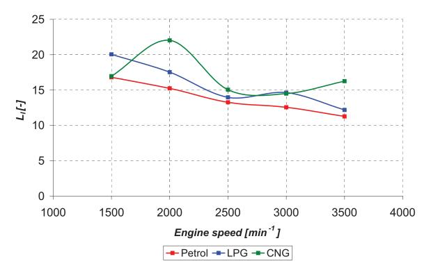
Fig. 13. Clearance factor of engine block vibration signal as a function of engine speed (full load)
