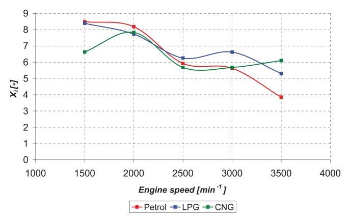
Fig. 11. Impulse factor of engine block vibration signal as a function of engine speed (full load)
