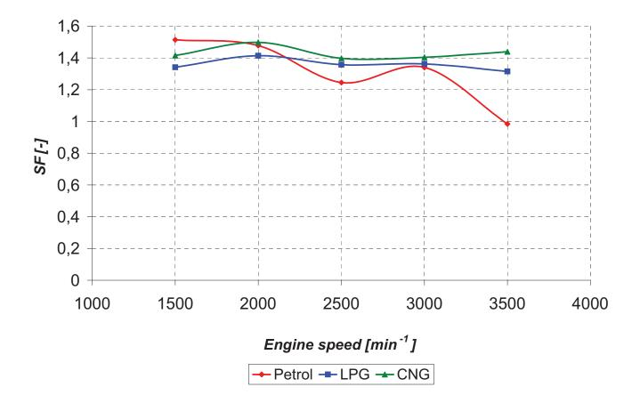
Fig. 10. Shape factor of engine block vibration signal as a function of engine speed (full load)
