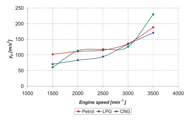
Fig. 6. Peak value of engine block vibration signal as a function of engine speed (full load)
