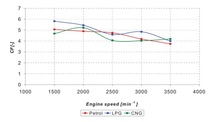
Fig. 9. Crest factor of engine block vibration as a function of engine speed (full load)
