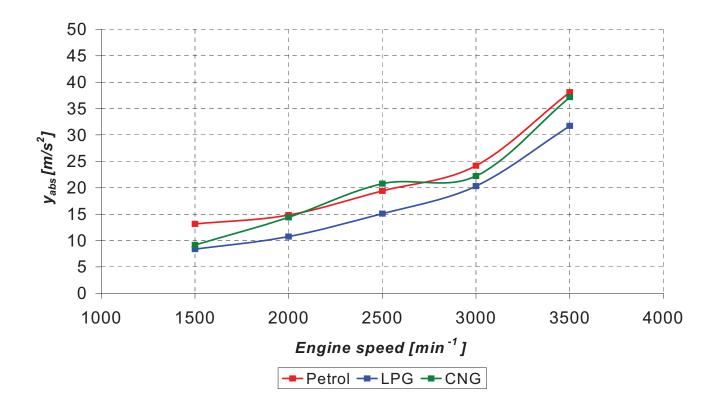
Fig. 8. Average mean value of engine block vibration signal as a function of engine speed (full load)
