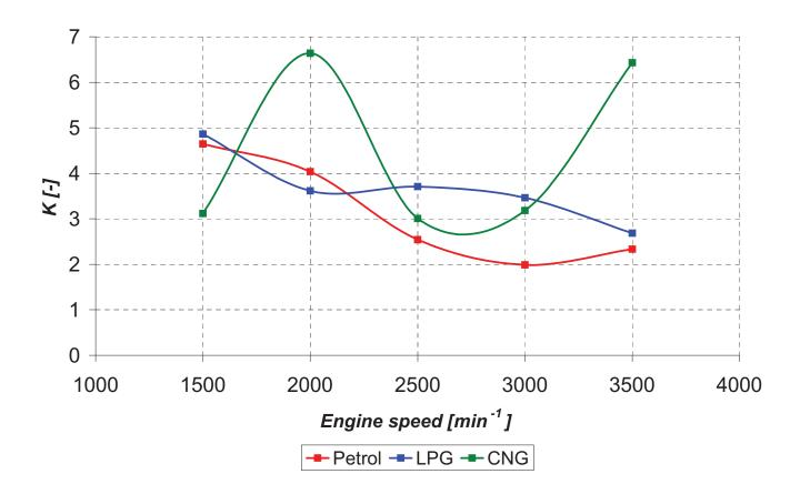
Fig. 12. Kurtosis of engine block vibration signal as a function of engine speed (full load)
