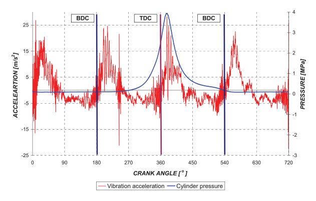
Fig. 5. Traces of fourth cylinder pressure and vertical vibration for engine fuelled by CNG (rpm=1500, full load)
