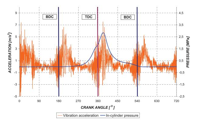
Fig. 4. Traces of fourth cylinder pressure and vertical vibration for engine fuelled by LPG (rpm=1500, full load)
