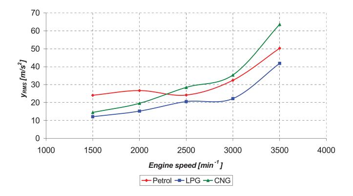
Fig. 7. RMS of engine block vibration signal as a function of engine speed (full load)
